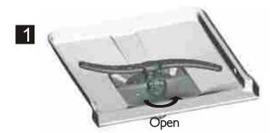
Step 1LTurn the filter in anti-clockwise direction.
